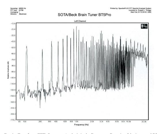
Fast Fourier Transform (FFT) Spectrum Analysis in the Frequency Domain of the improved BT5pro
