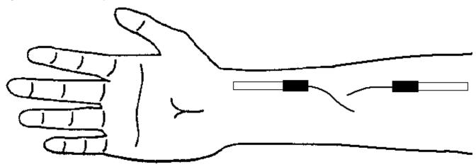
This figure illustrates the placment of the two electrodes on the same forearm and wrist. Position probes about 6" apart on the same Radial Artery.
